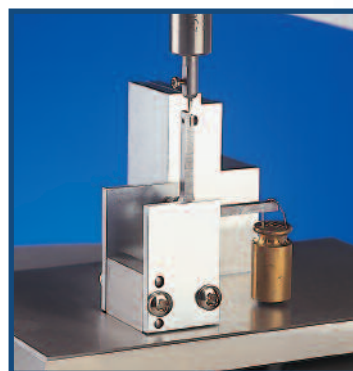
Automatic load cartridge calibration using traceable weights.
